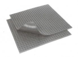
The smooth edge design of the low cost oil-resistant UNISORB NEOPRENE PAD prevents oil, grease, and dirt from accumulating beneath the load-bearing surface of the pad. Available in 18" x 18" x  $^{5}/_{16}$ ". Stiffness is 60 Durometer.
